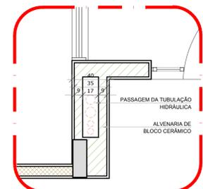
2 DETALHE - SHAFT HIDRÁULICA ESCALA 1/20
